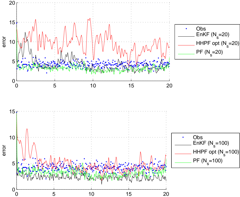
FIG. 9. Sparse observations, comparison of estimation errors of the EnKF, PF and optimized HHPF with observation error.
